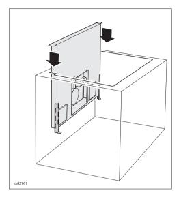
■ With the assistance of another person, lift the appliance into the prepared cutout. The top mounting brackets should rest on the countertop.
